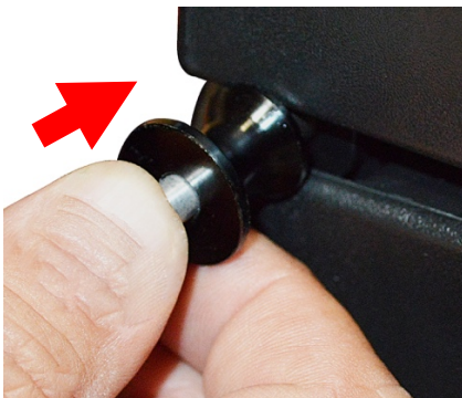
Secure front of top Imperio speaker to top of bottom Imperio speaker using Linkpin 1 .
